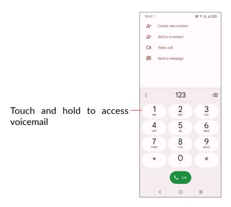
Enter the desired number from the dial pad and touch on to place the call or select a contact from **Contacts** or **Call logs** by touching tabs, then make the call.
