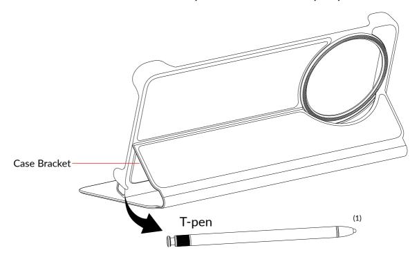
The button on the top of this pen is a physical button that helps you connect it to, or extract it from, the protective case.
