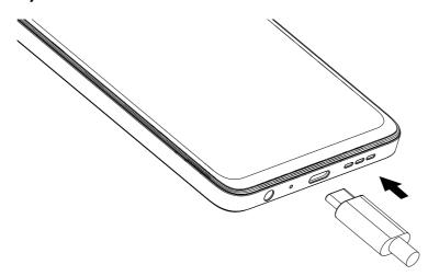
You are advised to fully charge the battery ( ). Charging status is indicated by a percentage displayed on screen while the phone is powered off. The percentage increases as the phone is charged.
