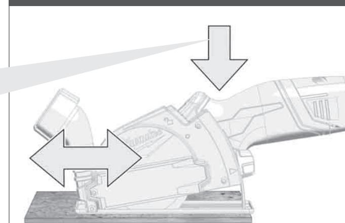
Adjust the cutting depth to the thickness of the workpiece.
